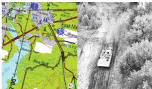
Split-screen (SS) mode displays two input signals simultaneously as equally sized images that are stretched/cropped to fit each window.
