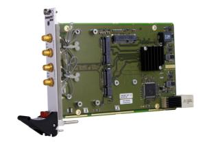
The G227 is a rugged single slot CompactPCI Serial carrier board for up to three PCI Express Mini Cards. It provides connectivity solutions to cellular networks by adding LTE, UMTS, GSM or other types of wireless modems. Each modem slot is equipped with two RP-SMA antenna connectors / cables by default. Other types of antenna connectors are available on request.
