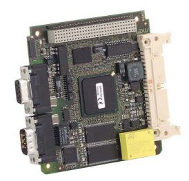
CAN interface can be located on SA-Adapters™ or on the carrier board. The board also features a real-time clock and watchdog.
