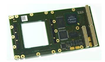
USM Universal Submodules make PMC modules more flexible than ever. The conduction-cooled main PMC P598 gets its specific function through the IP cores implemented inside the onboard FPGA. This function can be changed at any time through implementation of different IP cores. The corresponding line drivers are realized on the USM which is simply plugged on the P598.
