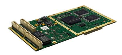
The P522 is a 32bit/33MHz PMC module with AFDX/ARINC-664 functionality. AFDX is a reliable, high-speed data bus commonly used in airborne applications for sending information between avionics subsystems. Its most important features are high data integrity, redundancy and deterministic behavior.
