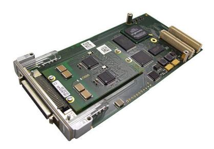
The P511 is a 32bit/33MHz PMC with dual Ethernet functionality. The two channels can be accessed via two RJ45 connectors which are led to the front via an adapter cable from a SCSI connector. They support half duplex and full duplex operation.
