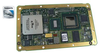
The MM1 is an ultra-small Computer-On-Module of the rugged ESMini<sup>™</sup> family. Together with an application-specific carrier board it forms a semicustom solution for industrial, harsh, mobile and mission-critical environments.
