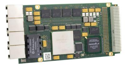
The EM9 is a complete embedded SBC for use on any carrier board in different industrial environments. The final application consists of a stand-alone EM9, an EM9 with an application-specific carrier card and/or with additional PCI-104 modules.
