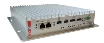
The BC50I is a maintenance-free box computer that has been designed for independent use or as display computer electronics for use in industrial applications, e.g. for machine control, surveillance or commercial vehicles or robotics.
