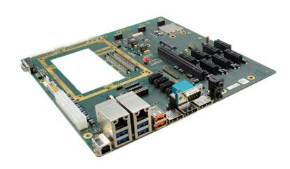
Rugged COM Express®, based on PICMG standard COM.0 or COM Express®, has been developed for demanding embedded applications with extended requirements for thermal design, shock, vibration and EMC. Rugged COM Express®, together with an application-specific carrier board, forms a semi-custom solution which is suited for application in extremely harsh, mobile and mission-critical environments.
