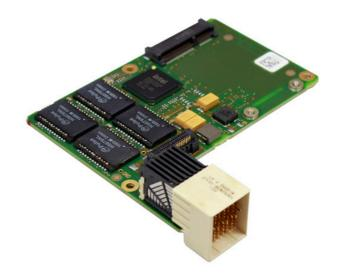
The GM3 is a mezzanine card which is plugged onto CompactPCI® Serial CPU boards to implement four Ethernet interfaces on the backplane.
