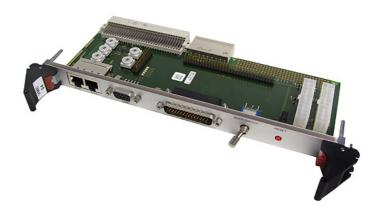
The CT15 is a 6U VMEbus transition module for use in combination with MEN's A602 single-board computer.
