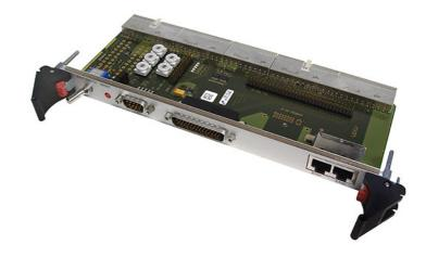
The CT14 is a 6U CompactPCI® transition module for use in combination with MEN's D602 single-board computer.
