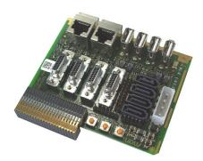
The CT12 is a 3U CompactPCI® rear I/O transition module for use in combination with MEN's PICMG 2.30-based single-board computers.
