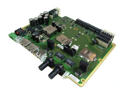
The AE51 is a combined graphics and I/O interface board for MEN's display computer electronics like the SC24 SBC and possible subsequent models.
