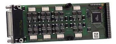
The mezzanine card M82 is a 16-channel fully isolated input M-Module with latching and comparator capabilities for industrial applications. A current limit for each input guarantees an input voltage range of 0 to 40 V. Each input signal edge generates a maskable interrupt for each channel. The voltage-sensitive inputs have a hysteresis function.
