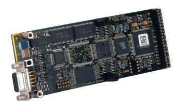
The mezzanine card M79 M-Module is a Profibus DP (Distributed Peripherals) slave interface based on the Infineon C165 CPU. It is thus an ideal interface solution for intelligent remote I/O applications via a very popular fieldbus standard.
