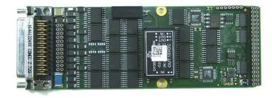
The mezzanine card M62N is an analog output device with as many as 16 channels on one single M-Module. The isolated supply voltages are generated by an onboard DC/DC converter. The output voltage range is programmable to 0 to 10 V or -10 to +10 V. Alternatively, current outputs are available within a range of 4 to 20 mA. The output load is driven to ground.
