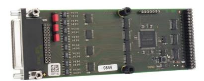
The mezzanine card M58 is a TTL I/O M-Module which is used for fast and trouble-free transmission of binary signals. It is organized in four 8-bit groups, where each group can be programmed as an input or output. Every group supports active termination, which can be activated by software.
