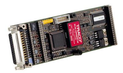
The mezzanine card M50 is a 1-channel, continuous-tracking synchro- or resolver-to-digital converter with a configurable 10 to 16-bit resolution and a tracking rate of up to 1040 rps. The M-Module has a reference signal generator with a frequency range of 50 Hz to 20 kHz. Reference output voltages can be in a range of 2 Vrms to 21 Vrms. An analog velocity output can be used to monitor the rotational speed.
