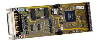
The mezzanine card M47 is a Serial Synchronous Interface M-Module for connection of up to four sensors to optically isolated SSI outputs. Serial synchronous interfaces are commonly used for many kinds of sensors such as rotary encoders. Connection to the sensors is made by two signals - a transmit clock and a receive data signal.
