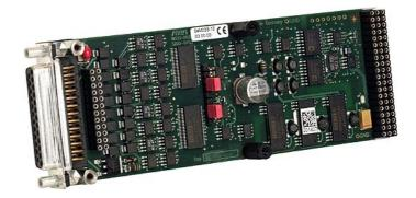
the current outputs can be used with 0..20mA or 4..20mA. The output load is driven to ground.
