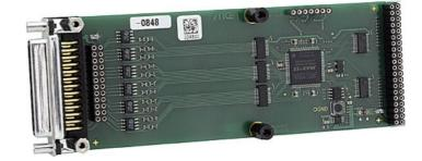
The M11 mezzanine card is a TTL I/O M-Module with 16 lines (Ports A and B) that can be used separately as two ports with 8 bits each or together as a 16-bit port. Control of the I/O lines is via the four handshake lines.
