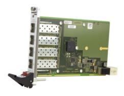
The GP2 is a 3U Gigabit Ethernet PHY line card implemented as a CompactPCI<sup>®</sup> Serial board. It occupies one peripheral slot using a 4 HP front panel with four Gigabit Ethernet ports on SFP cages.
