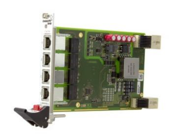
The GE1 is a 3U Gigabit Ethernet line card, with optional PoE support, implemented as a CompactPCI® Serial board. It occupies one peripheral slot using a 4 HP front panel with four Gigabit Ethernet ports on RJ45 connectors. Alternatively, the GE1 can be supplied with four M12 connectors on the front panel (X-coded variants in preparation).
