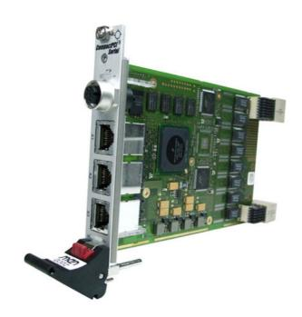
The G302 is a managed 3U Ethernet switch implemented as a CompactPCI® Serial board. It occupies one system slot or one peripheral slot, using a 4 HP front panel with 3 Gigabit Ethernet ports on RJ45 or M12 connectors and one service interface via M12.
