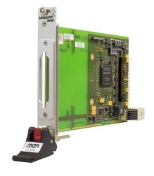
The G204 is a 3U M-Module carrier board for universal I/O on the CompactPCI<sup>®</sup> Serial bus. It allows high flexibility in applications such as data acquisition or process control.
