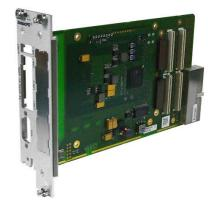
slot can be used for 32/64 bit and 33/66 MHz PMC cards and supports up to 133 MHz PCI-X. The board detects automatically whether an XMC or a PMC is plugged.
