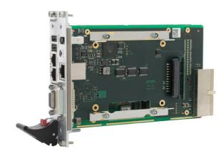
The F604 is a 4HP FireWire and multimedia extension card for 3U Intel® based CompactPCI® single-board computers. It can be used in combination with the F14 and compatible CPU boards. The IEEE 1394 high-speed serial bus is often used in combination with modern high-end digital camera equipment instead of USB. Thus, the F604 side-card extends the standard features of a powerful multi-core or Pentium® M CPU board by one 400 MBit/s FireWire interface connected via PCI
