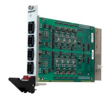
Its voltage range from 14.4 VDC to 154 VDC and its current output of 1 A at 24 V complies with EN 50155, which makes the board ready for immediate use in train applications.
