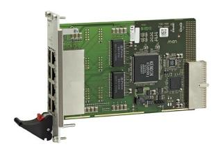
The F301 is an unmanaged 3U Fast Ethernet switch module with a maximum of 8 channels at the front panel (8 RJ45 or 6 D-Sub connectors) and an integrated Fast Ethernet controller. The Ethernet switch is an unmanaged device, meaning that it is not recognized by other CompactPCI® devices thereby removing the need for additional software. As an option it is also available as a fixed managed device, with a customized, hardware-coded configuration.
