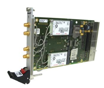
The F223 is a rugged single Eurocard CompactPCI® carrier board supporting the PCI Express® Mini Card standard.
