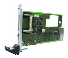
The F217 is a 3U 4HP CompactPCI® board which offers a multitude of memory configurations. It is equipped with a CompactFlash® socket and a multi card reader which supports MS, SD and MMC plus cards.
