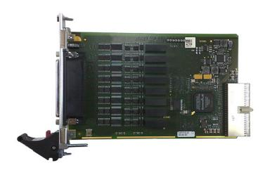
The F216 is an octal UART I/O board based on 3U CompactPCI®. Two UART controllers provide four full-duplex serial channels each. The physical layers are integrated on the board: each of the eight channels can be individually configured as single-ended RS232 or differential RS422 or RS485. The default setting is RS422.
