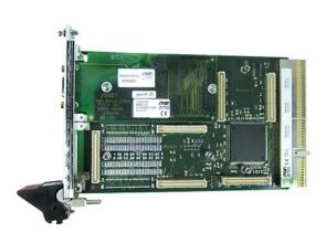
The F203 is a 3U PC-MIP® carrier board for universal I/O on the CompactPCI® bus. You can install up to three PC-MIPs on the F203, with two Type I/II PC-MIPs and one Type I PC-MIP®.
