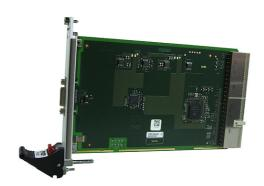
The F100 is used in combination with the G100 to connect a CompactPCI® Serial system to a CompactPCI® system. The CompactPCI® Serial backplane and the CompactPCI® backplane can either be located in one housing or in two separate ones. The F100 is plugged into the system slot of the CompactPCI® system. It is equipped with a PCI-Express-to-PCI bridge which acts as a master for up to 7 PCI devices. It supports 32-bit and 33-MHz.
