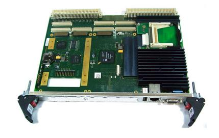
on the A20. One x1 PCIe<sup>®</sup> link is used for the onboard Ethernet interface, three x1 links support the XMC slots, one x1 link supports the PMC slots via a PCI Express<sup>®</sup> to PCI-X bridge and one x1 link is used for connection of the VMEbus bridge. The PMC slots support 64bit/66MHz (PCI-X).
