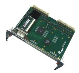
The A15C is a PowerPC® MPC8245 based single-board computer for embedded applications. It features full VME64 support and it can be used as a master or a slave in a VMEbus environment. The A15C provides 1 MB local dual-ported SRAM for slave access and communication between the local CPU and another VMEbus master.
