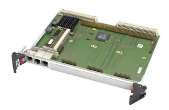
The A15B is a PowerPC® MPC8245 based single-board computer for embedded applications. It features full VME64 support and it can be used as a master or a slave in a VMEbus environment. The A15B provides 1 MB local dual-ported SRAM for slave access and communication between the local CPU and another VMEbus master.
