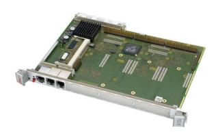
The A12B is a single-board computer for embedded applications based on the PowerPC® MPC 8245. It can be used as a master or slave in a VMEbus environment or as a stand-alone card. The A12 provides up to 1MB local dual-ported SRAM for slave access and communication between the local CPU and another VMEbus master.
