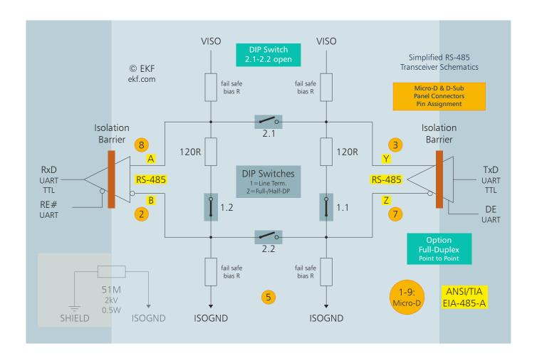
Illustrated above is a point-to-point 4-wire configuration (in addition to reference ground wire). Switches 2.1 and 2.2 are open. Setting of line termination switches 1.1 and 1.2 depends on data transfer bit rate and cable length. Normally set both switches on (off if external termination is applied).
