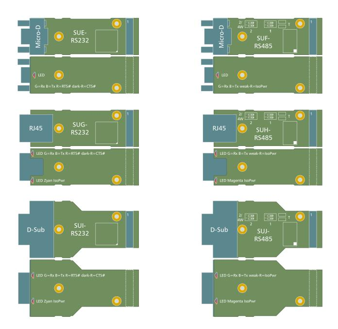
The SUE-SUJ transceiver modules are provided with one ore two tri-colour signal LEDs, located at the PCB bottom side. The LEDs will be visible through suitable front panel cutouts. Their meaning varies according to the illustration above. Please note that the front panel view depends also on the mounting orientation of a particular transceiver module - component side down or up.
