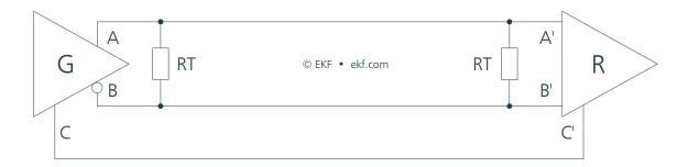
G = Generator • R = Receiver • RT = Termination Resistor
