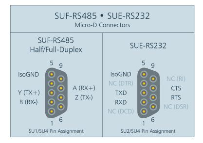
IsoGND is the reference ground for all signals of a particular I/O connector, isolated from the board and system logic GND, and from Shield (panel/chassis), and also from other transceiver modules.
