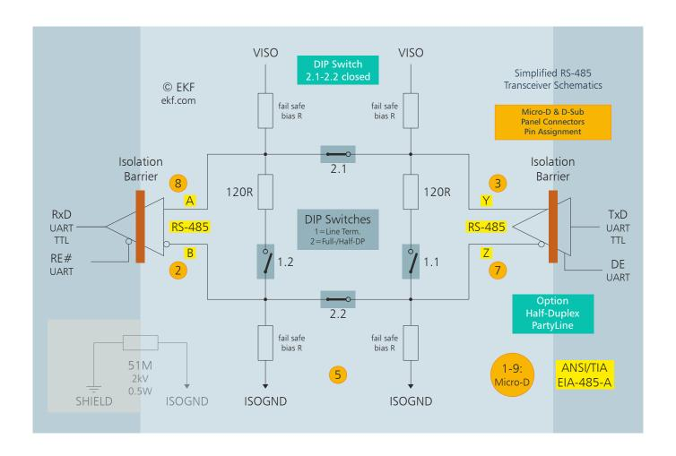
On a PartyLine bus, no more than a single node is allowed to send data at a particular time; all other nodes must disable their drivers in order to avoid data collision at the same time. A suitable software protocol must be established which controls the driver enable (DE) pin of the transceiver. The SUx-RS485 were designed for the Pericom/Diodes PCIe<sup>®</sup> to UART bridge, which requires proprietary driver software for DE control.
