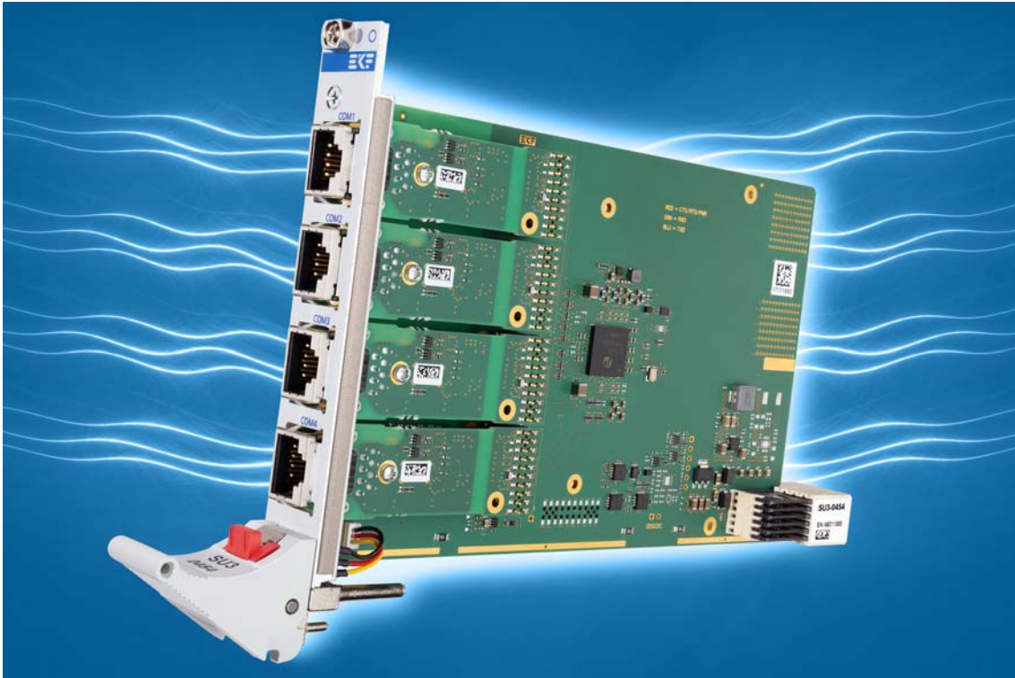
SU3-045x-ENSEMBLE w. 4 x RJ45 Transceiver Modules (4HP Front Panel)
