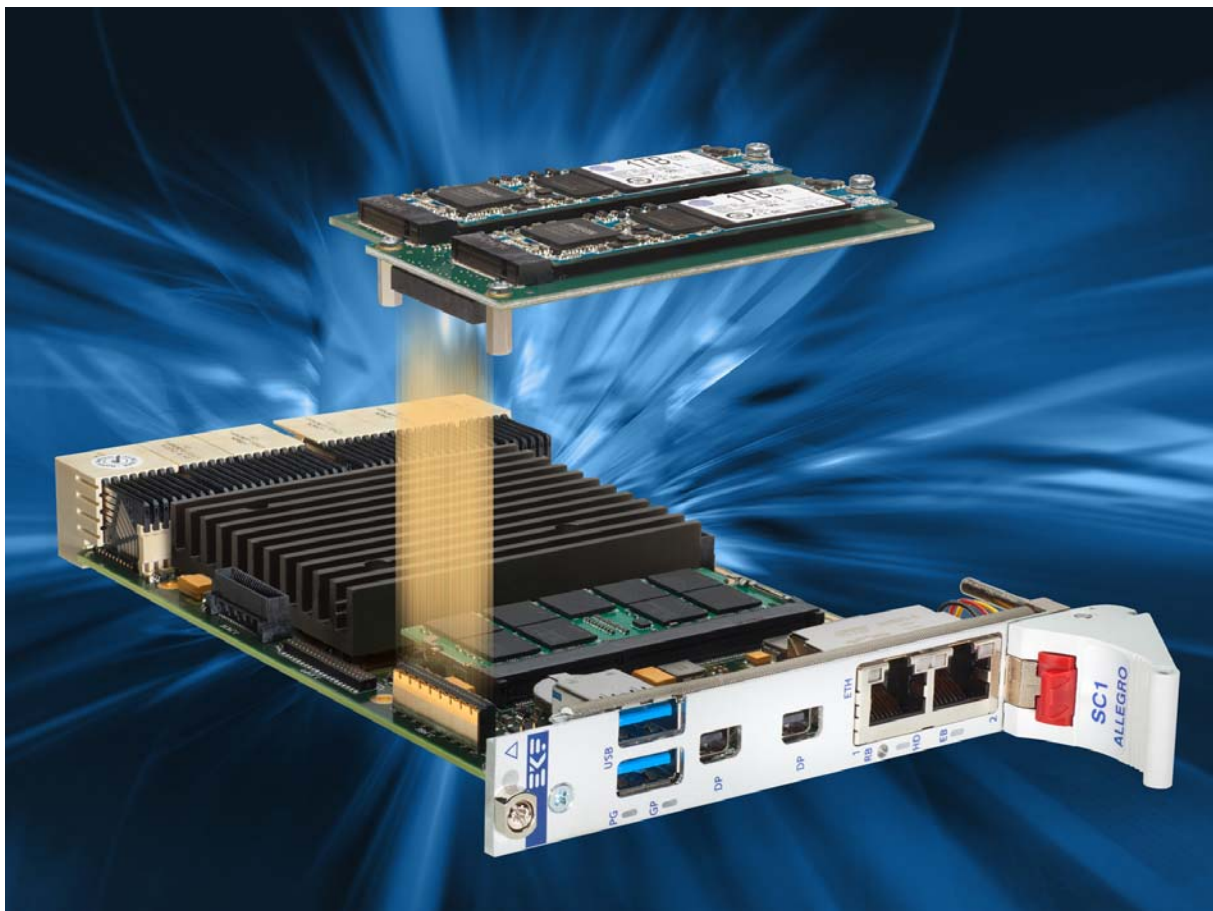
C48-M2 over CPU Carrier Card (4HP Assembly)
