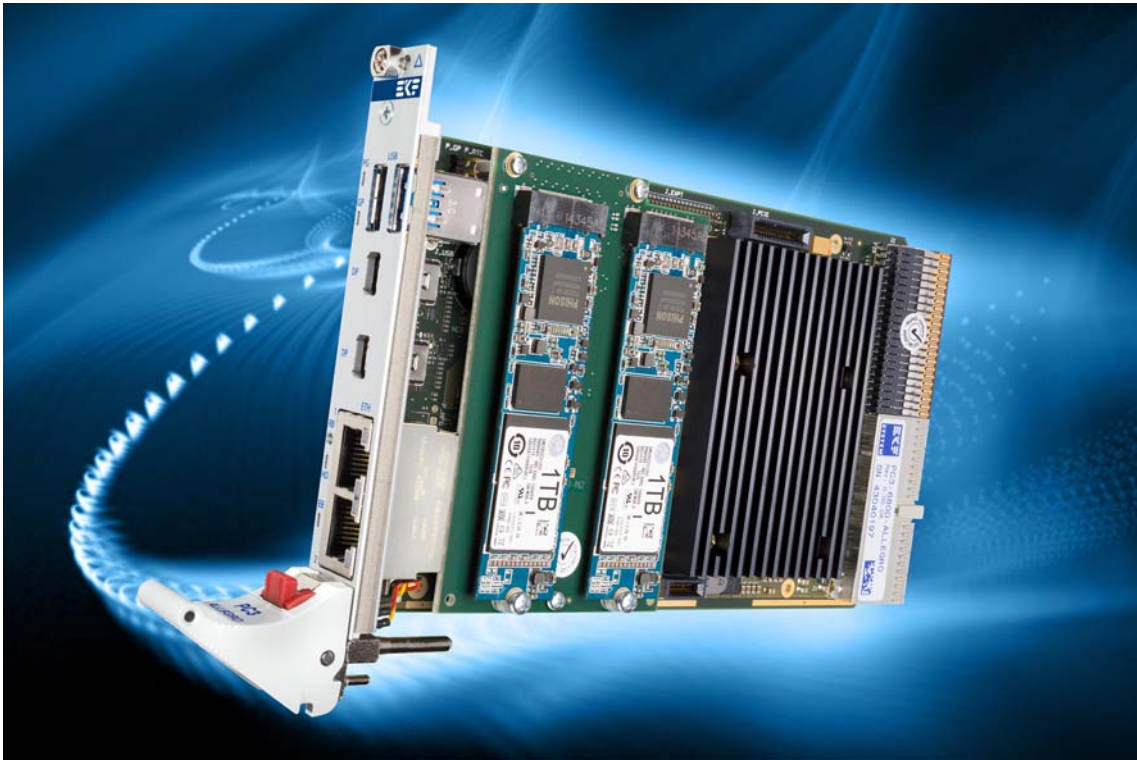
C48-M2 Mounted on a CPU Carrier Board (4HP Assembly)
