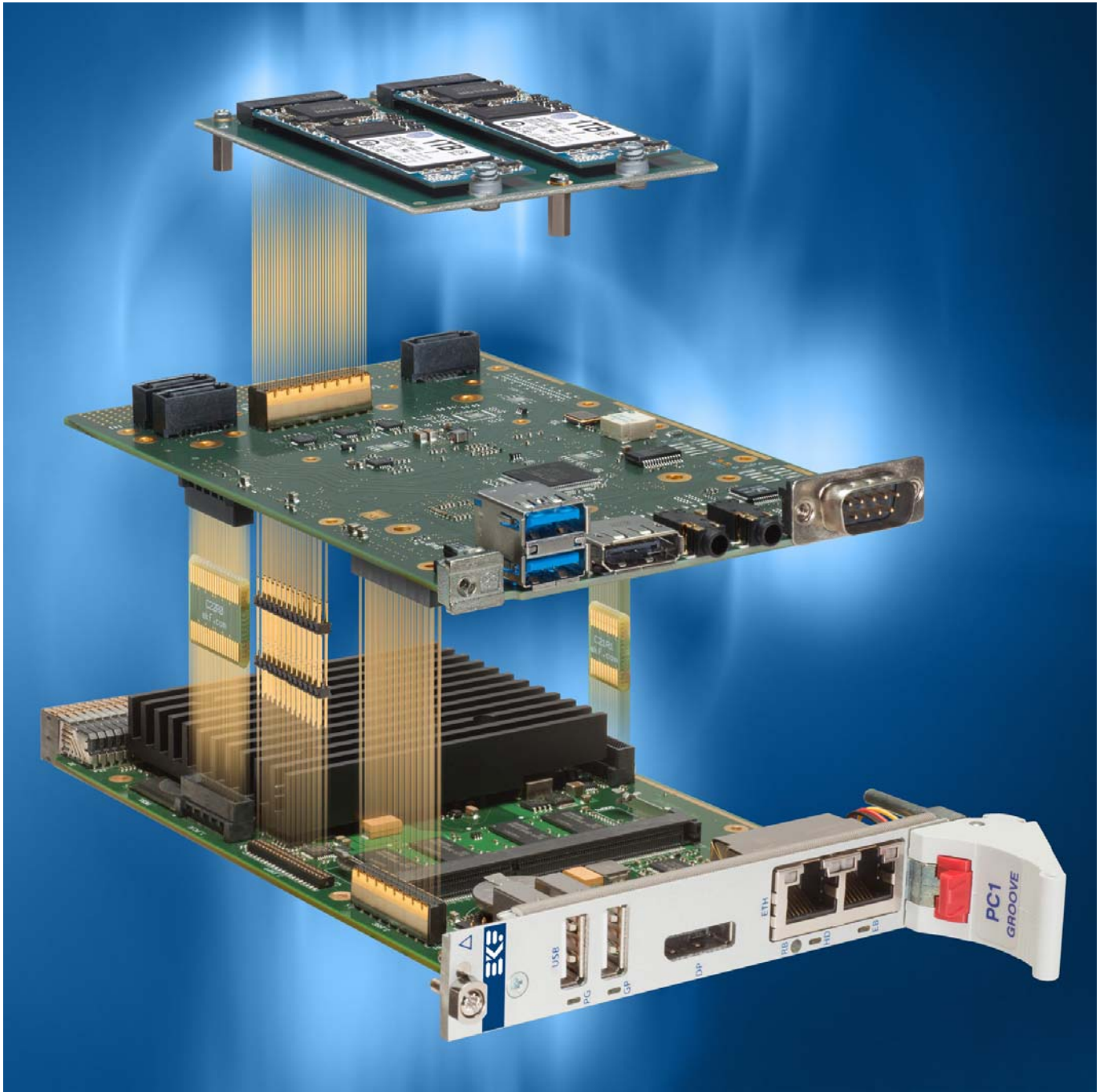
C48-M2 Mounted on a Mezzanine Side Card (8HP Assembly)
