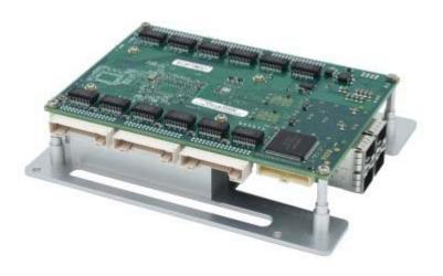
EPS-24G4X Ethernet switch with conduction cooling used in SabreNet-24000
