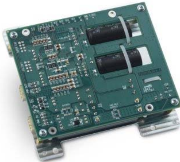
Top view showing power supply mounted on conduction cooling mounting plate
