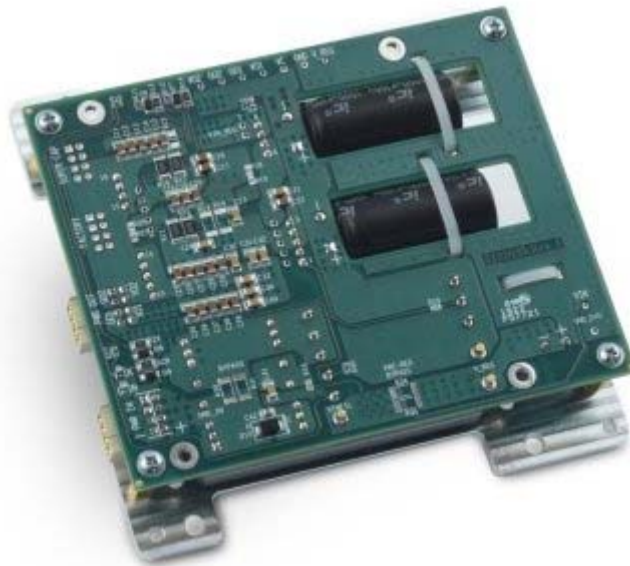
Assembly view with conduction cooling mounting plate
