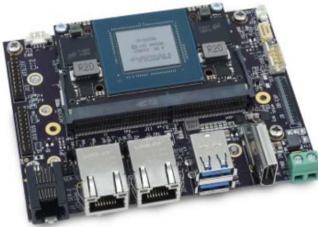
Jackson with Orin NX installed
