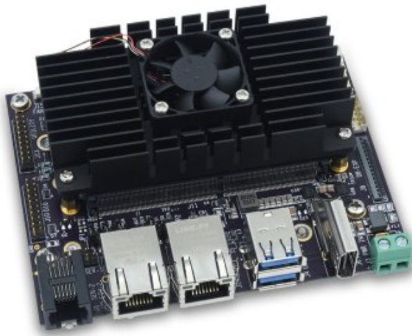
Full system assembly with Jetson and fan sink
