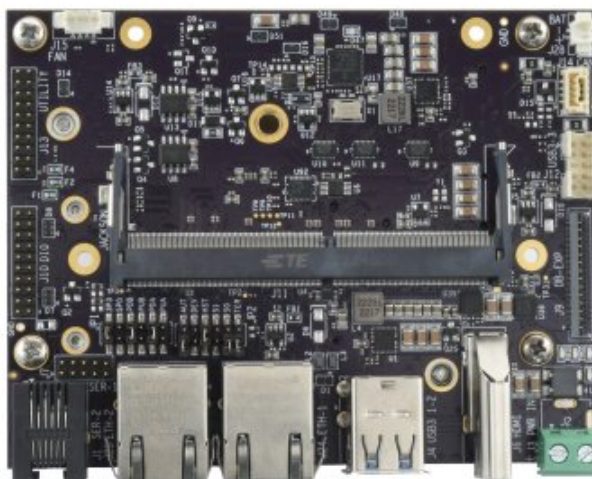
Top view with Jetson socket and I/O
