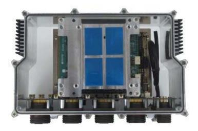
Bottom view showing optional conduction cooled MIL-grade power supply with filtering
