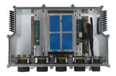
The entire system is housed in a rugged 3-part enclosure that eliminates all T joints and includes seals at all joints to ensure IP67 compliance.
