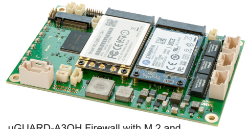
μGUARD-A30H Firewall with M.2 and 2x mPCIe, with WiFi & additional Flash (115 x 75mm)
