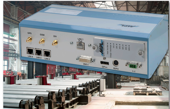
PIP38 used in harsh environments, equipped with UPS and removable battery, GPRS, GPS, and PoE.
