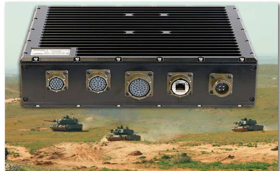
MIL-PIP32 for rough use in military environment as communication controller.
