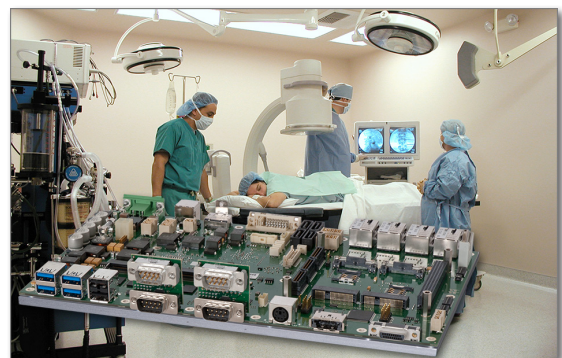
OPEN-PIP31 for integration in existing housing. Cooling plate & CPU board are semi-customized.
